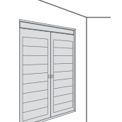
Reveal fixed inside the window door reveal
